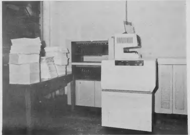
Stacked copied material and collated sets can be done rapidly and efficiently on the new machine which can print 120 copies per minute. At left are the Sorters.
